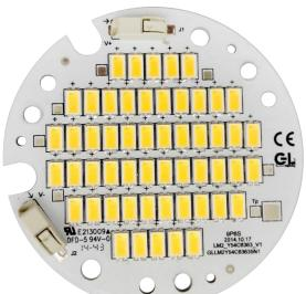
The maximum allowed temperature at the  $T_p$  point of the board is 80°C. This temperature is not based on the LM-80 standard but is for warranty purposes only.
